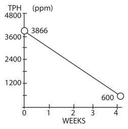
29 Palms did not disc or add any additional water to the contaminated soil for the next four (4) weeks. <u>NOTE:</u> Our instructions specify to disc the soil at least once a week and keep the soil at a level of approximately 30% humidity.
